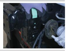
Set the winch support bracket in place making sure the wiring harness is routed below the bracket as shown.
