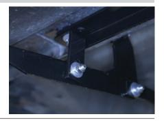
Locate the rear driver-side mounting holes.
