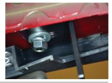
Locate the driver-side rear mounting point. Insert a 60mm flag-bolt plate into the opening. Slide a plastic bolt retainer over the thread of the bolt to hold the bolt in place.
