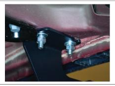
Locate the driver-side middle mounting point. Insert a 60mm flag-bolt plate into the opening. Slide a plastic bolt retainer over the thread of the bolt to hold the bolt in place.
