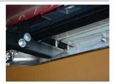
Attach the running board to the brackets using six M8 bolts, lock washers, flat washers and nuts.
