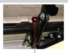
Drill 7/16" hole for 8mm rev nut
