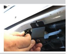
Measure rivet nut hole locations on the Z-hanger brackets. The center-to-center distance should be approximately 7 7/16". Adjust as needed.
