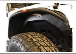
Using an M6 bolt, M6 flat washer, and M6 lock washer, attach the outer fender flare (if used) to the top support brace on the Jeep.
