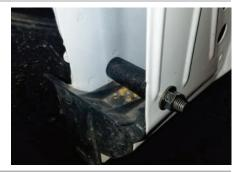
Place the fender back into place and secure using an M6 bolt, lock washer and flat washer.
