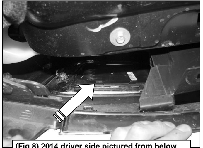
(Fig 8) 2014 driver side pictured from below front bumper. Carefully pull the air dam slightly forward and reach up between bumper cover and radiator support to access and remove block offs
