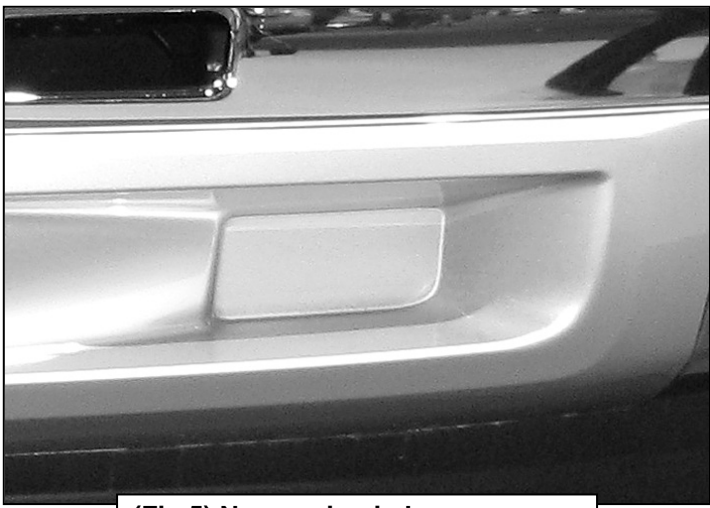
(Fig 5) No opening in bumper cover
