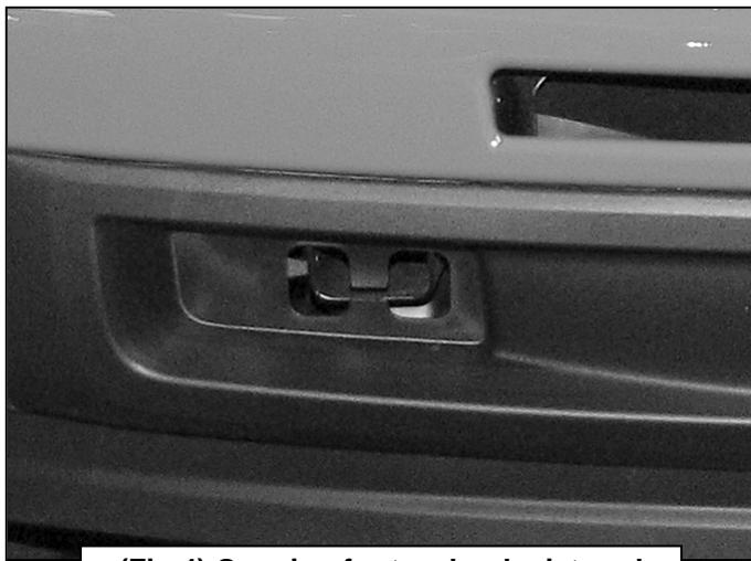
(Fig 4) Opening for tow hook pictured
