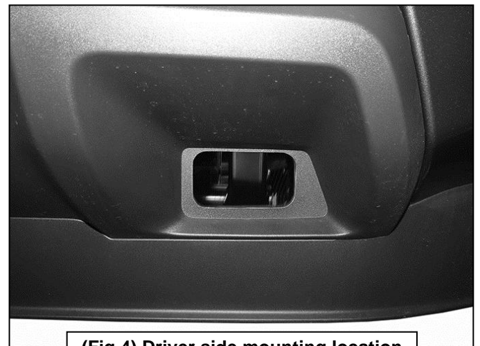
(Fig 4) Driver side mounting location
