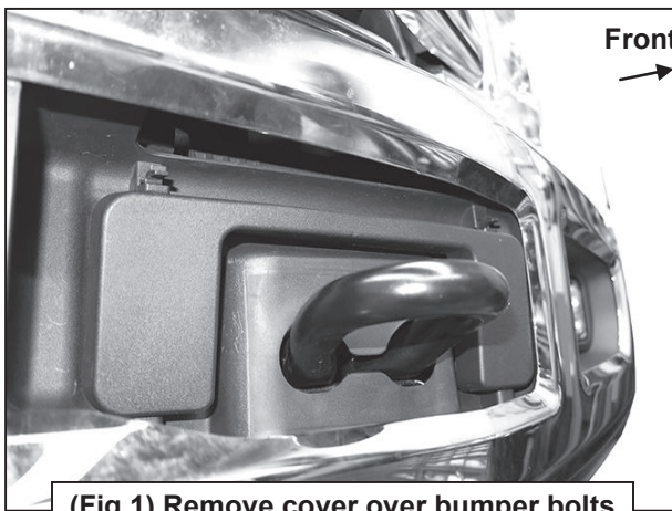
(Fig 1) Remove cover over bumper bolts
