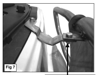
8mm x 20mm Button Head Bolt 8mm Lock Washer 8mm Flat Washer 8mm Hex Nut
