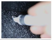
If one of mounting points do not line up with a factory hole, mark a new mounting location. Drill a new hole at the marked location using a 11/32" drill bit. Check to make sure that the threaded metal insert will fit.
