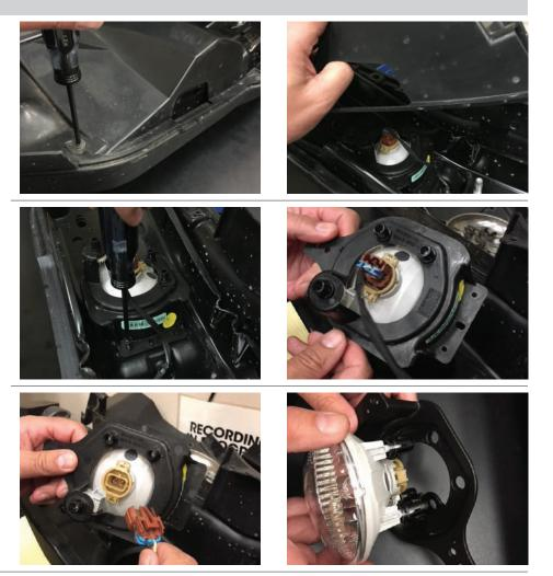
Remove the fog light wiring harness from the factory bumper. Begin by removing the retainer clips from the eight bumper mounting studs.
