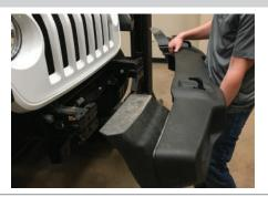
On the driver side, remove the plastic cover over the factory fog light. Remove the fog light and plastic housing from the factory bumper.
