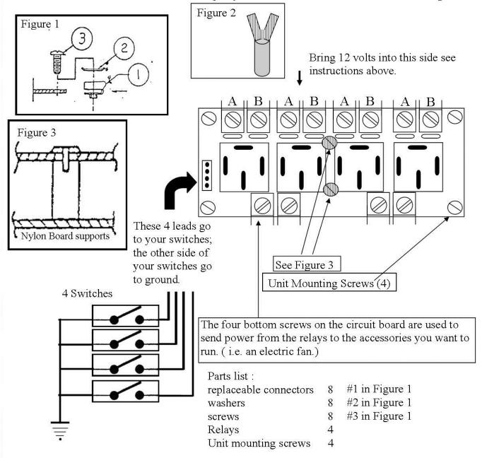
Strip wire back 3/8 of an inch and insert under washer and tighten screws.
