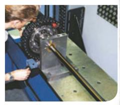
ARB's locker test rig statically tests the Air Locker's strength against the axle. ARB tests both standard and aftermarket axles, with our goal being to always have the axle break before causing damage to the Air Locker.
