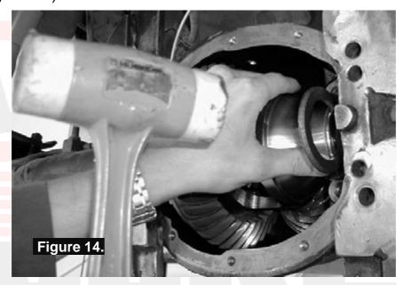
NOTE: If the shim pack is too tight to fully install then the spreader tension may need to be increased. <u>Do not spread the housing more than 0.50mm [0.020"].</u>
