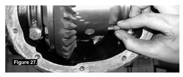
Completely remove the long cross shaft.
