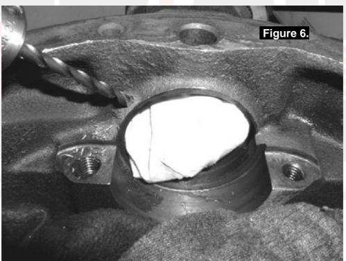
NOTE: Cover the differential housing cavity and the axle tube openings with a rag to protect them from metal filings.
