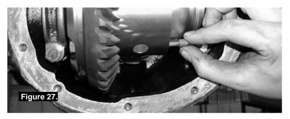
Completely remove the long cross shaft.
