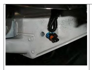
11. If vehicle is fitted with fog lights, remove globes from sockets and cable tie fog light loom to vehicle panel.
