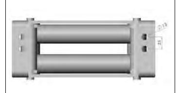
24. Drill two new 13mm holes in the roller fairlead provided in the kit, as shown on the adjacent picture.
