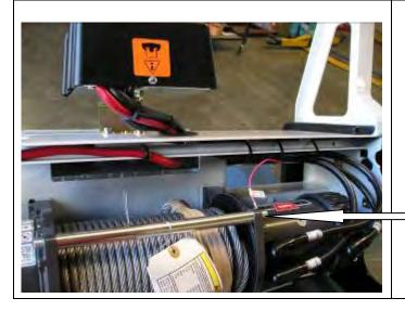
32. Fit all 3 cables to their correct terminals and tighten. Refer to Warn installation instruction when wiring up winch. Fit plastic boots over terminals. Cable tie cables to brace as per photo to clear of all moving parts. Fit ground wire under winch tie rod. ( See Photo )
