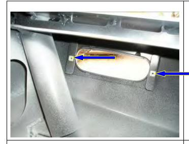
14 Fit white nylon plugs into square holes in light bracket.
