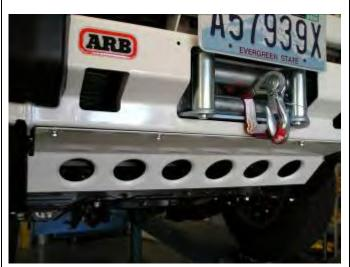
38. Fit splash pan to lower flange of bull bar using M6 x 20mm bolts, 6mm spring washers and 6mm large flat washers.
