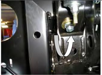
8. Secure from underneath using large 12mm gold coloured flat washer,12mm spring washer and M12 nut to both sides of vehicle.
