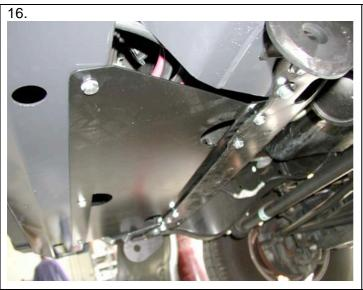
Bolt the air deflector to the underside of the bar and chassis cross member using M8 bolts, M8 flat washers and M8 spring washers.
