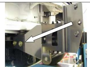
7. Mount the Impact Absorber brackets to each side of the chassis using original fasteners.
