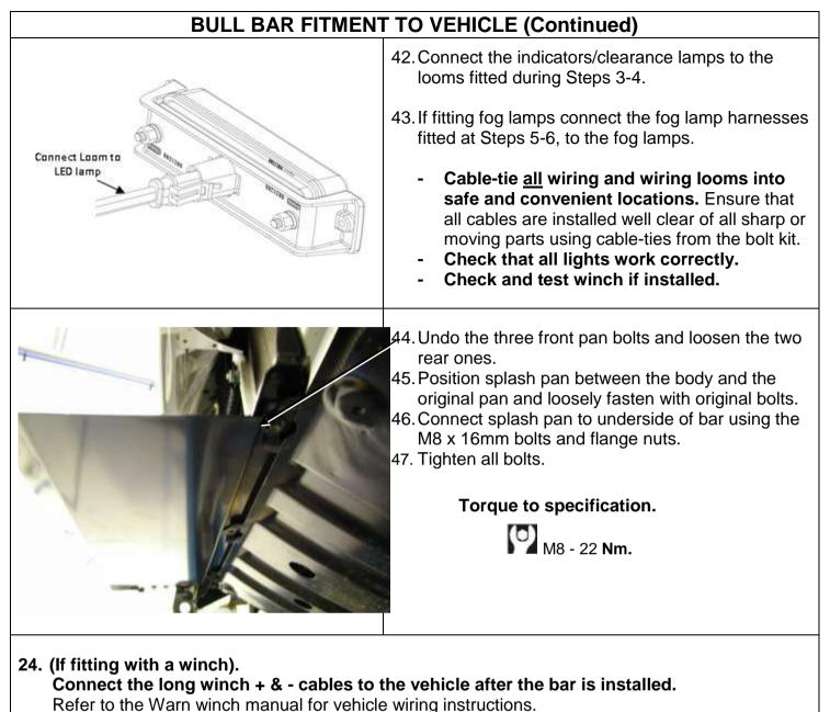
Ensure that these cables are installed well clear of sharp, hot or moving objects. Secure the winch cables to the vehicle and winch bumper with the supplied cable ties.
