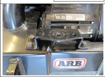
If driving lights are to be used fit left and right driving light mounts now using M8 x 25 bolts, M8 spring washers, M8 flat washers and M8 flange nuts.
