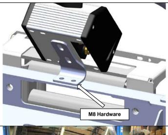
15. If mounting a control box on the bar secure mount to bar using M8 x 25 bolts, M8 spring washers, M8 flat washers and M8 flange nuts. Secure control box to bracket using manufacturers' hardware.
