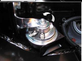
9. On 3.6 V6 models the horn is mounted on the right hand side. Remove the nut mounting the horn to bracket and place horn on opposite face. Rotate horn by hand until sitting horizontal as shown in the image. Trumpet must be facing towards winch mount. Tighten nut when complete.
