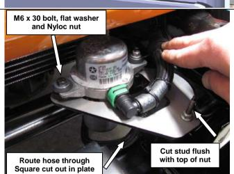
Un-bolt vacuum pump and place new mount 8. on chassis as shown. Orientate pump as shown and mount using original nuts on studs and M6 x 30 bolt, flat washer and Nyloc nut on opposite rubber mount. Secure piping using cable ties in kit. NOTE: Cut stud flush with top of nut.
