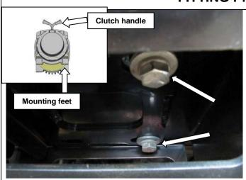
10. Make sure winch clutch handle is facing upwards (opposite mounting feet). If using Warn ZEON or CTI winch use 8mm thick packers and longer 3/8 bolts supplied. Carefully place winch into bar (winch motor on RH side) and secure with hardware supplied with winch through access holes placed in front and rear of bar. Secure to manufacturers torque settings.
