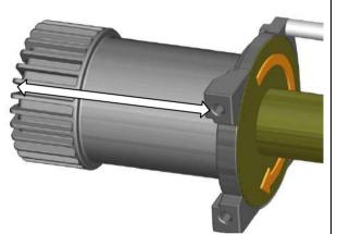
If fitting a winch measure the distance between winch mounting hole and the end of the motor. If this distance is greater than 172mm then a notch in the chassis flange must be cut. Follow step 4.
