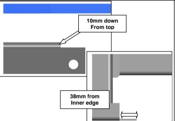
Measure from top RH front of chassis down 10mm and mark a line. Measure from inner edge towards chassis centre 38mm and mark a line. Cut this section out using a grinder with cutting disk, de burr and paint.
