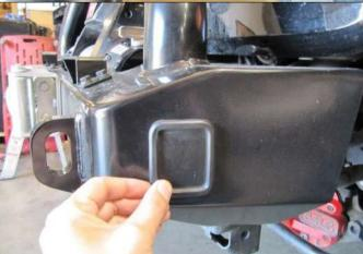
18. Fit high lift jack plugs to bar.
