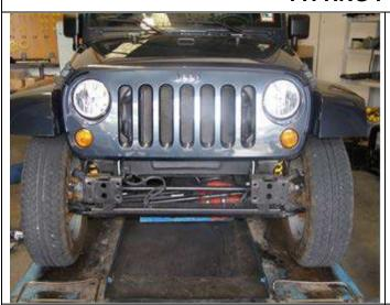
2. This is how the vehicle must be prepared before fitting a bar to the vehicle. Wrap up and cable tie fog light wiring (if fitted) out of the way.
