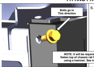
Place bar onto vehicle and secure inner mounts using M10 SEMS bolts and M10 flange nuts. Nuts to be placed towards front of vehicle. Make sure vehicle horn is re-fitted, 3.8 V6 on LH side and 3.6 V6 on RH side.
