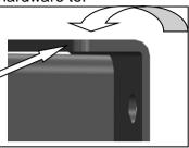
Insert spanner Into high lift Jack hole
