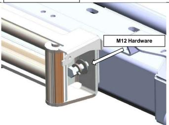
14. Place winch cable through fairlead and sandwich license plate mount between fairlead and bar. Secure using M12 bolts, flat washers, spring washers and M12 nuts.
