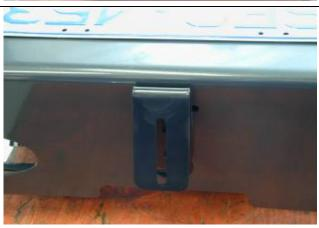
27. Fit the control box bracket to the bull bar using two M8 x 20mm bolts, M8 flat washers and M8 flange nuts.
