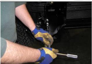
15. Fit the chassis mount bracket to the chassis using the original flange nuts removed with the bumper reinforcing bar. Centre the chassis mount bracket and tighten.
