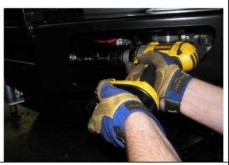
35. With the bull bar in position drill Dia10mm pinning holes, one though pilot hole in mount bracket and one through hole in upright for both sides of mounts.
