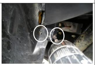
59. Drill 7mm securing holes in the liner and the plastic bracket arm as shown.
