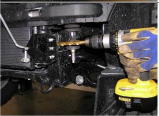
8. Using the 13mm drill bit and power drill, drill out the M8 captive nut located at the outboard side of the chassis as shown, on both sides of the vehicle.
