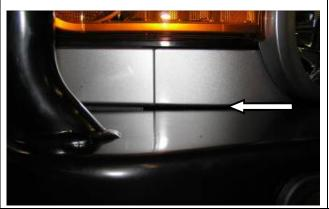
34. Position the bull bar so that there is an even gap of approximately 5mm from the top face of the bar to the underside of the body edge. Then tighten all the bolts.
