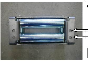
19. Using a 12mm (1/2") drill bit, drill two new holes in the roller fairlead 25mm below the original holes.
