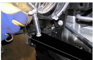
32. Fit supplied replacement brace and secure with original fasteners
