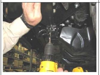
If there is <u>no</u> corresponding hole in chassis brace lower flange to fix inside flange of the wing under panels....
