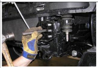
Check that the nut body is completely removed, if it is not cleared, using a cold chisel and hammer chisel the remainder off.
