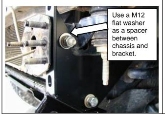
11. Fit the chassis mount braces to the vehicle using the M12 x 30mm fine pitched bolt, M12 spring and flat washers supplied in the lower hole. Use an M12 flat washer as a spacer between the brace and the chassis at the upper hole and fix with an M12 x 40mm bolt M12 spring and flat washers and M12 x 1.75 nut. **Do not tighten the bolts.**
