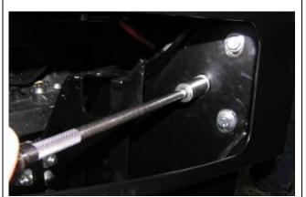
33. With the help of an assistant position the bull bar on the chassis bracket and fix with six M10 x 30mm bolts, M10 spring and flat washers.
