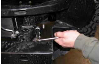
7. Remove front bumper reinforcing bar.
