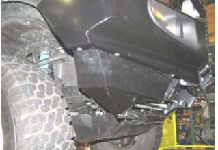
49. Fit the wing under panels as shown using M6 bolts and washer sets to bolt to wing
