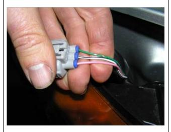
39. Wire up lights using loom extensions supplied in fitting kit.
