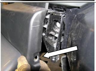
6. Remove screw then remove front bumper cover from vehicle.
