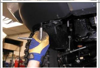
3. Remove lower bumper fixing screws and screws in wheel arch area
