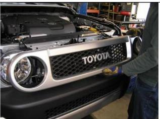
4. Remove grille. Screws are located in tabs at top of grille. Once these are removed carefully release clips some are located along the inside lower section.
