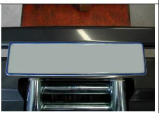
30. Insert square grommets into holes in front of bar for licence plate fixing. Place the doublesided tape along the top edge of the number plate. Using supplied black Hi-lo screws, attach the licence plate to the bull bar.
