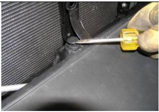
5. Remove plastic rivets along top of bumper
