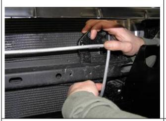
16. If required, carefully bend A/C piping clear of mount bracket assembly as shown, with <u>a</u> minimum clearance of 20mm (3/4").
