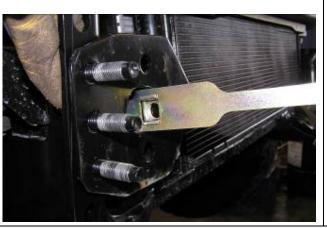
12. Insert the captive nut assembly through the front of the chassis and line it up with the hole at the end of the mount brace. Fix in place with the M12 x 1.75 x 40mm bolt, M12 flat and spring washers. Break off the end of the captive nut plate. Do not tighten yet.
