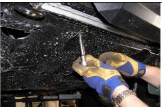
2. Remove front fasteners only from stone tray. Retain fasteners for reuse.
