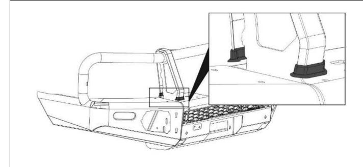
54. Place each of the front buffer sections onto the bar as shown. Ensure that the 2 lugs and 2 screw bosses pass through the holes in the bar and that the buffer sits flat against all surfaces,
