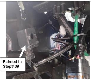
73. Once satisfied that sturdy electrical connections have been made on both sides, cable tie both harnesses back onto the sheet metal underneath the headlights as shown.
