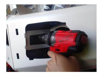
86. Using the M10 pilot holes in the bull bar uprights, drill the two pinning holes through mounting brackets on each side. Fit M10 bolt and washer sets and flange nuts and tighten to specified torque.
