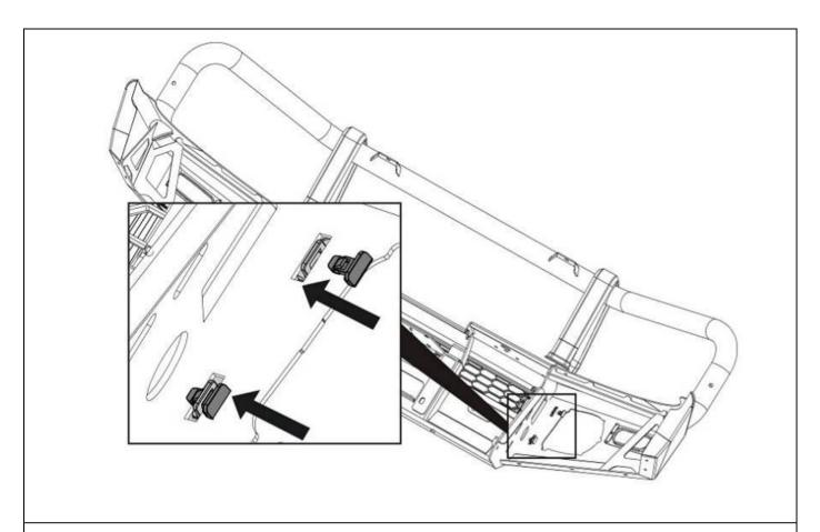
57. From the rear of the bar slide the rear buffer sections into the front sections as shown. Ensure the tongue section on both sides of each buffer engages into the slots of the front sections.
