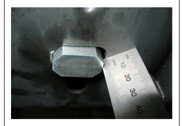
82. Then tighten up the long M12 chassis studs, ensuring that the clevis nut is positioned correctly over the hole in the chassis.
