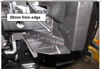
34. Mark out and trim the air deflector on the LHS of the vehicle using a Stanley knife or similar.
