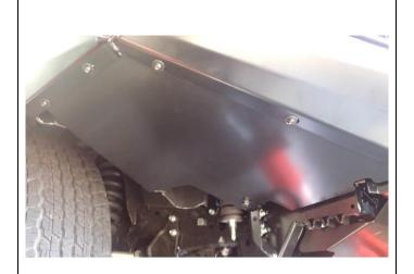
100. Trim the fender liner end flush with the splash panel face as shown. Then tuck the remaining wheel liner inside the wing panel return.
