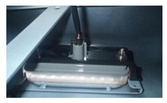
92. Connect indicator looms to combination LED Indicator/Clearance light.
