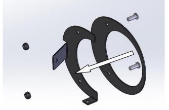
88. Assemble Fog Shroud and Retaining bracket with M6X16 Button head bolts and Nyloc nuts as shown adjacent (RHS). NOTE: Notch in shroud at top
