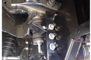
Fit both wing panel brackets to the higher holes in the outside of the mounting brackets using M8 bolt, washer, spring washer and flange nut.
