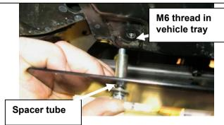
94. Fit stone tray using 4 x M6 bolts and washer sets at front under bull bar and 2 x M6 x 40 bolts, washers and 18mm long tube spacers at two locations into existing sump guard front section as shown.
