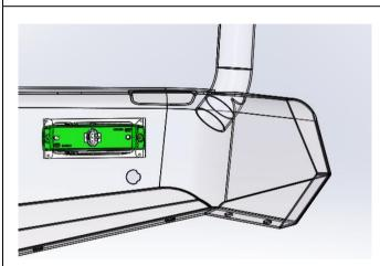
59. Fit the small plastic grommets to the bar and attach the combination LED lamps to the bar using the screws provided with the lamp kit. Details provided in Fitting instruction 3789197.
