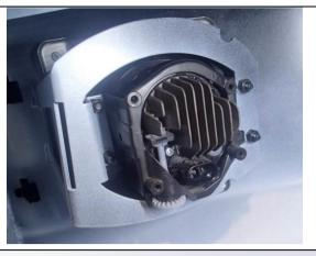
87. Install OEM LED Fog lights into bar from the front, using M6 button head bolts and nyloc nuts.
