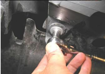
5. Remove lower bumper retaining screws.
