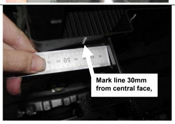
30. Mark the lower section of the air scoop for the power steering radiator as shown. This is for trimming to clear the mount brackets.
