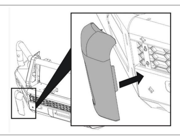
55. Attach the buffers to the front centre face of the bar using the angled cup washers and the screws provided.
