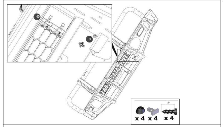
56. Attach the buffers to the front faces of the wings using the plastic clip provided.
