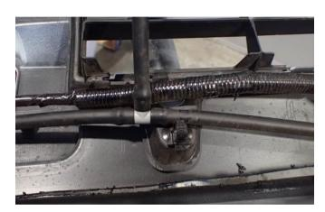
23. Remove OEM Fog lights, Parking sensors, washer lines and electrical loom from bumper, these will be reused. Label which side parking sensors are taken from for re-fitment.
