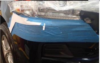
10. Apply wide masking tape along bumper as shown, then having cut out template; apply to outer corner of RHS bumper as shown. Align with edge of quarter panel, wheel arch and underside of head light.
