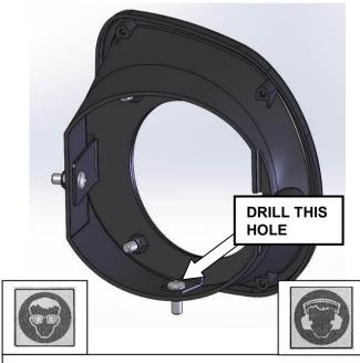
Warning: Drilling operations can result in flying metal debris, safety glasses should be worn.
