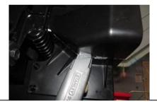
31. Now mark along the lower bend as shown, now cut the shroud along the marked edges as shown
