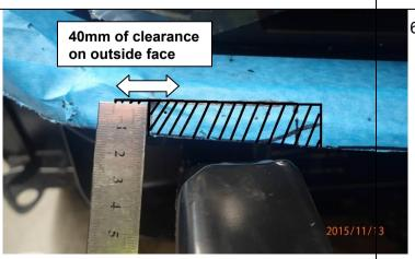
67. The Mounting brackets will contact the bumper, mark a rectangular cut on the bumper to ensure that there is a minimum of 25mm of clearance between the mounting bracket and the bumper. 40mm clearance is required on the outside face of the mount. Remove shaded area of bumper.
