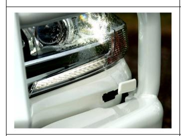
85. Check HLW Function; ensure there is adequate clearance between bull bar and extended HLW units.
