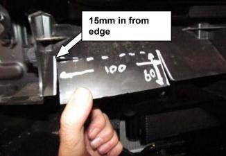
33. Now on the upper face of the power steering shroud mark and cut as shown
