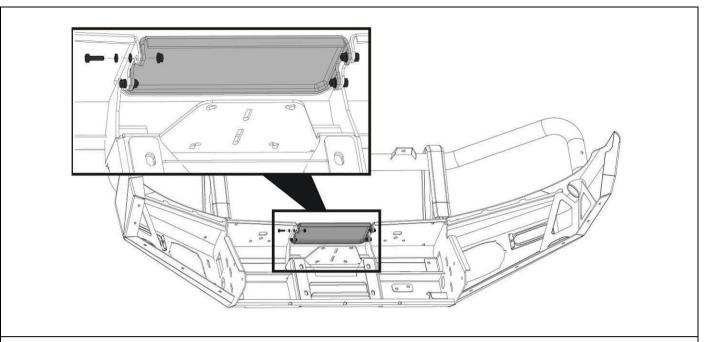
44. Fit the number plate bracket to the top face of the lower-centre pan on the bar using 3 x M6 x 20 hex bolts, spring washers, flat washers and flange nuts.
