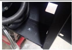
93. Fit the 4 longer leg M6 cage nuts to the lower pan of the bull bar as shown.
