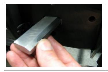
60. Insert clevis nut into rectangular hole in the inboard face of chassis, ensuring the threaded end is inserted first.
