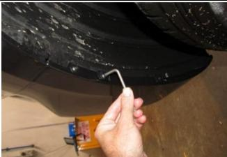
2. Remove inner guard bumper retaining screws three per side using T30 Torx key
