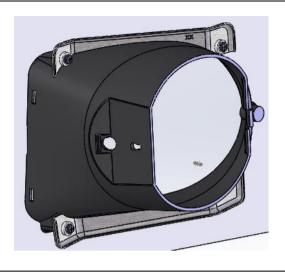
91. Install Foglight surrounds (p/n 3163156) as per instructions no. 3789552 supplied with surround kit into aperture of bull bar. Fog Shroud and Retaining bracket must be installed into modified surround.
