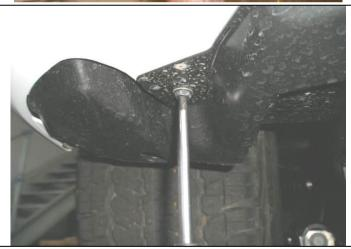
3. Remove lower trim panel sets each side which attach to bumper and engine protective plate area then set aside, they will not be reused.
