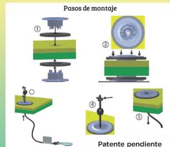
**WARNING!** ONE TIME SNAP ASSEMBLY ONLY, "DO NOT SNAP PARTS TOGETHER UNTIL ASSEMBLING ON THE FOAM PAD AS INDICATED IN THE DRAWING".
