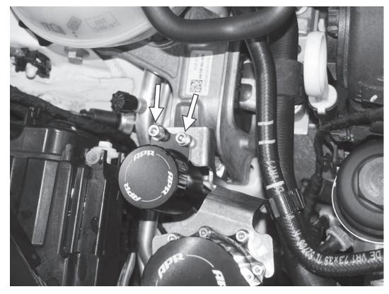
25) Mount the APR washer filling cap to the previously installed APR bracket with the two supplied 5mm allen screws. The washer fluid can be topped off if desiired.
