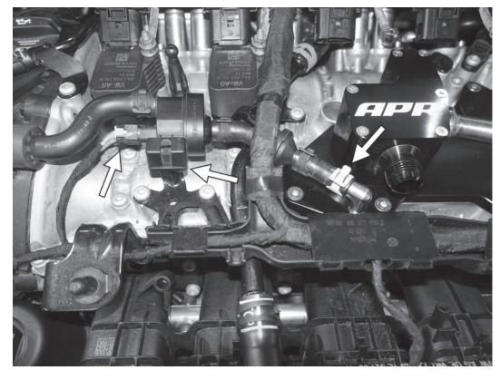
19) Connect the N80 hose to the port on the APR top plate. Secure with the spring clamp. Reattach the N80 valve to its original mounting bracket, and reconnect the electrical connector to the N80 valve.
