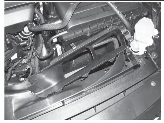
5) Lift the connection to the airbox inlet and remove this piece from the car.
