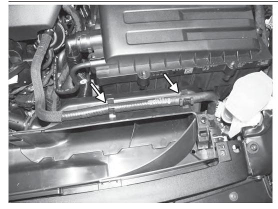
3) Carefully unclip the heater hose from the two tabs on top of the air scoop.
