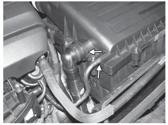
7) Remove the vacuum line from the front right corner of the factory airbox by pulling it off. Then, if equipped, remove the connection to the secondary air pipe by pressing down on both sides of the fitting and pulling away from the airbox.
