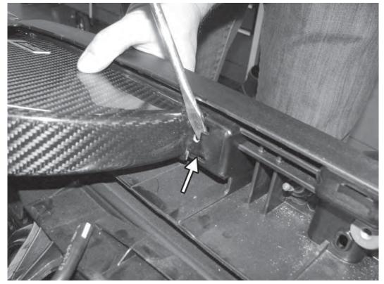
13) Loosely place the APR intake in the car. Slide the right mounting tab of the intake underneath the mounting point on the back of the factory radiator support. It may be necessary to carefully pry the factory tab back for the APR intake to fit. Once in place, slide the entire APR intake to the right side of the car to lock it in place.
