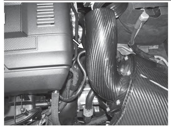
15) Connect the vacuum line that was on the right side of the factory airbox to the vacuum port on the bottom of the APR intake tube.
