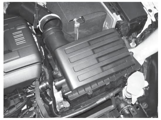
9) Carefully but forcefully lift up on all sides of the factory airbox. The airbox is mounted on three rubber posts underneath, and these must be popped off to remove the airbox from the car.
