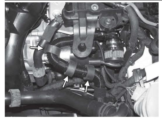
11) If equipped, adjust the three factory rubber bumpers on the secondary air pipe to keep the pipe from rubbing on the engine starter.
