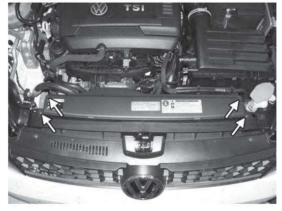
1) Remove the four T25 screws that hold the top cover of the factory air scoop.
