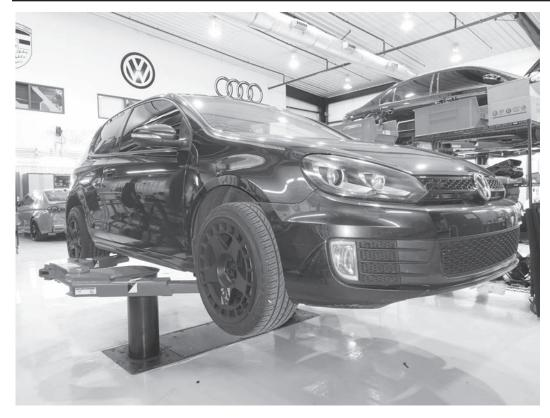
1) Securely lift vehicle. If a vehicle lift is not used, secure the vehicle with jack stands.
