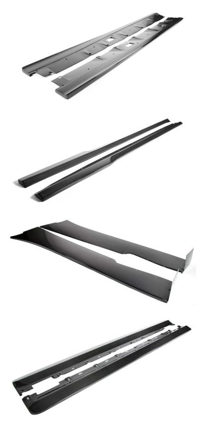
APR Performance Side Rocker Extensions, Rear Bumper Extensions, and Vertical Extensions, include mounting holes and all necessary mounting hardware.
