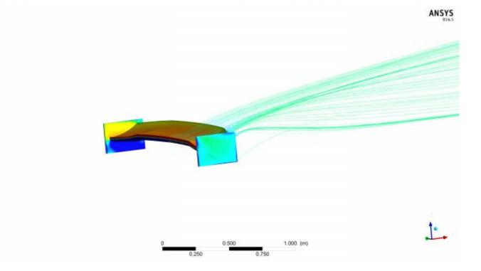
The following image illustrates both the pressure distribution on the underside of the airfoil
