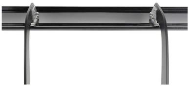
Supporting the airfoils are 10mm "aircraft grade" 6061 billet aluminum swan neck pedestals that come in a flat black powder coat finish. Each swan neck pedestal is also "knife-edged" at the trailing edge, to minimize the amount of "dirty" air that reaches the airfoil.
