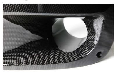
Other APR Performance Air Ducts are designed to exhaust hot air away from heat-sensitive areas.
