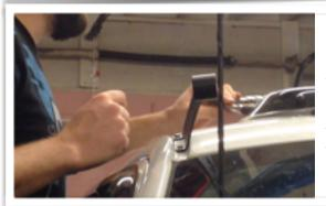
Install the roof mount brackets and leave the bolts a little loose to allow for adjustments while mounting the light bar. Apply silicone to the threads of the bolt to prevent water leaks. Get a second person to help hold the light bar while installing light bar mounting bolts. Tighten all mounting bolts, you may have to adust the angle of the light bar at dark to your needs. Depending on vehicle your power wire should be able to tuck behind the windshield trim.
