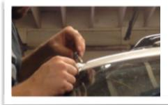
We prefer to snug the rivet nut on to the install tool and tap them into the holes. Using a wrench hold the install tool nut still and tighten the bolt till rivet nut stops spinning. Make sure the rivet nut is secure.
