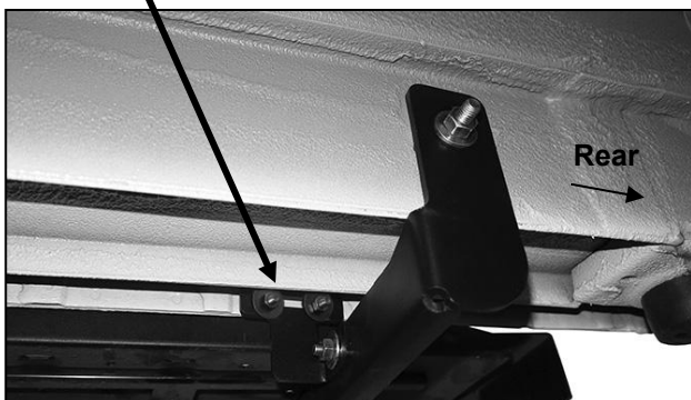
(Fig 15) Attach Support Bracket to pinch weld (passenger/right rear Bracket pictured) (For example only)
