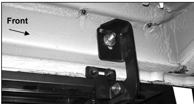
(Fig 18) Driver/left Front Brackets installed (For example only)
