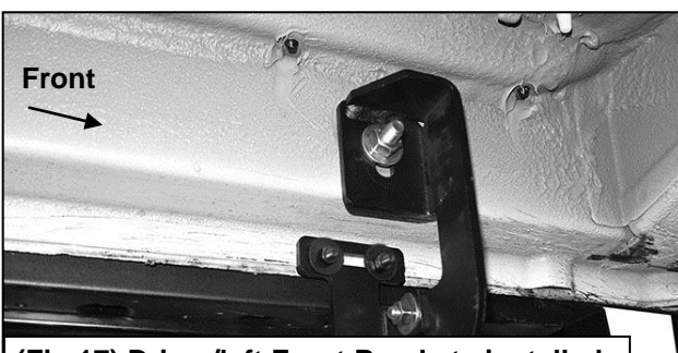
(Fig 17) Driver/left Front Brackets installed
