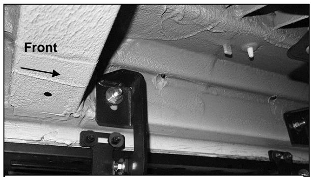
(Fig 18) Driver/left side rear Brackets installed
