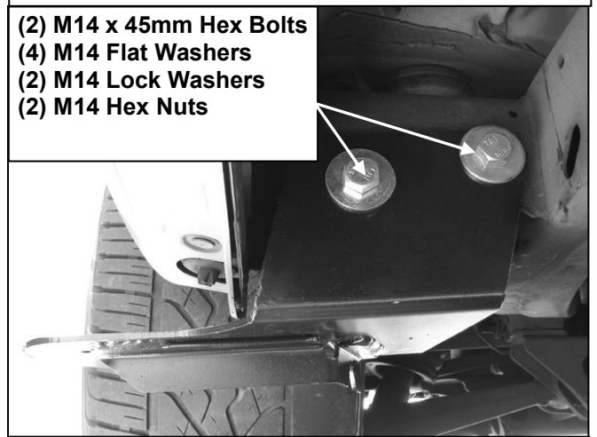
(Fig 9) Passenger side rear Mounting Bracket pictured after plastic cover removed
