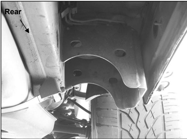
(Fig 4) Driver side rear body mount pictured after plastic cover removed
