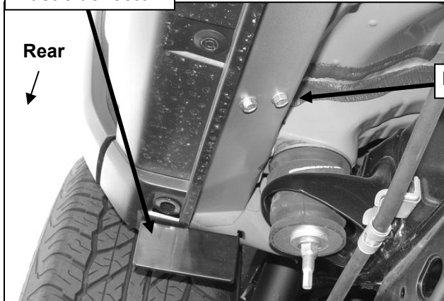
(Fig 3) Passenger side rear bracket location pictured
