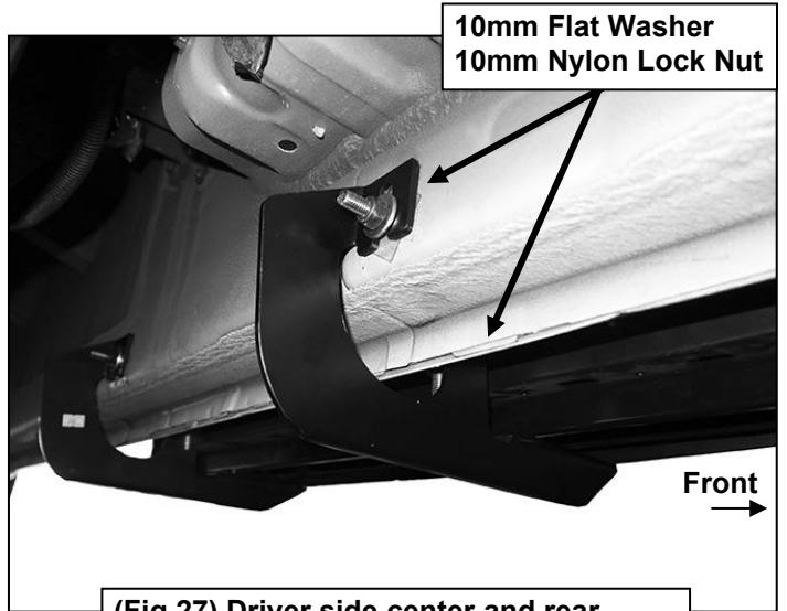
(Fig 27) Driver side center and rear Mounting Brackets completely installed
