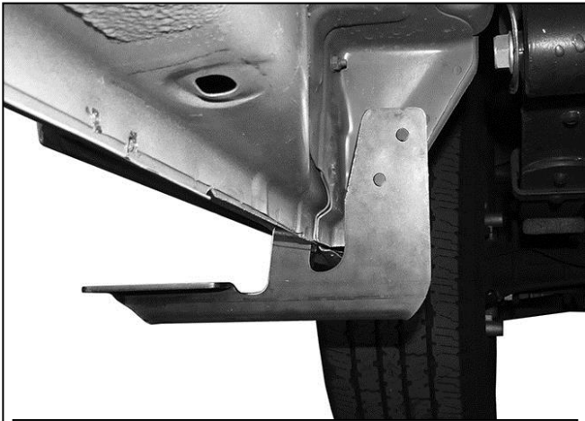
(Fig 14) Passenger side rear mounting Bracket
