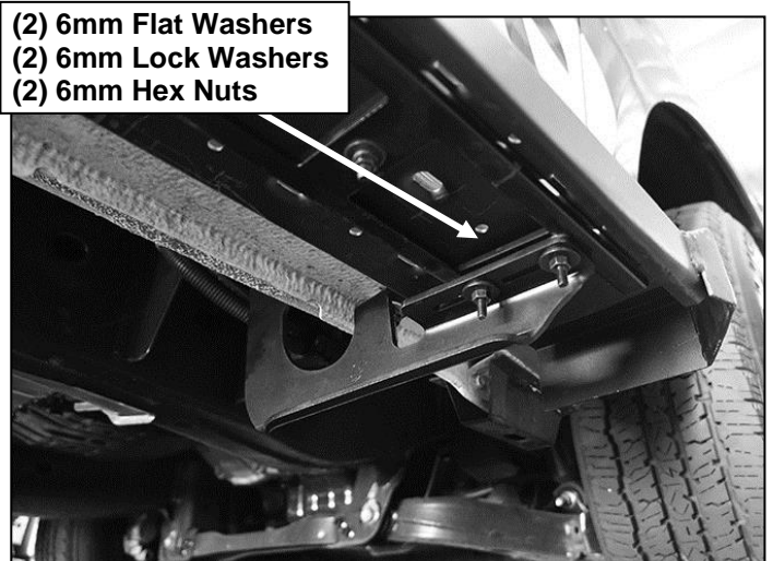
(Fig 17) Passenger front Bracket with Running Board
