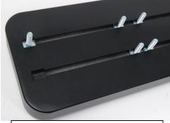
(Fig 4) Slip 6mm T-bolts into the bottom channel
