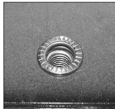
(Fig 11) Tighten Hex Bolt to collapse and lock Threaded Insert into factory hole
