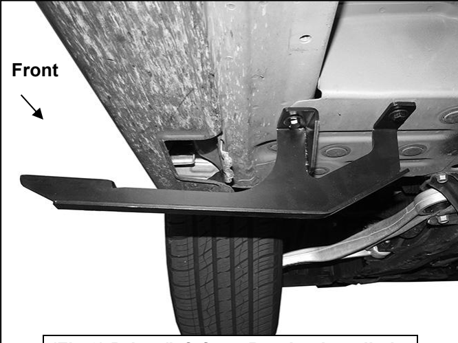
(Fig 3) Driver/left front Bracket installed
