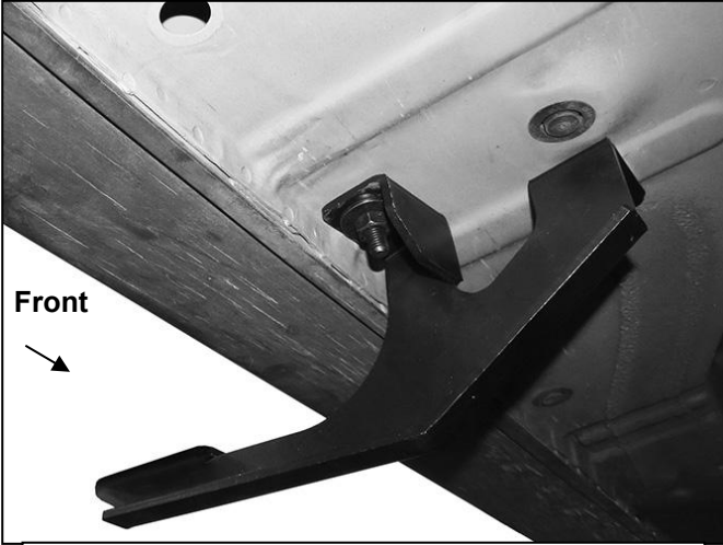
(Fig 7) Driver/left side Center Bracket installed
