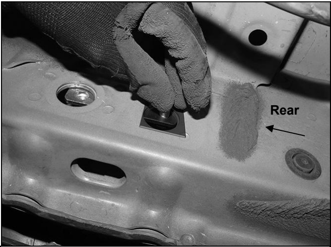
(Fig 10) Driver side rear mounting location. Insert 8mm Nut/Bolt Plate into round hole. Hold Bolt Plate and thread 8mm Plastic Retainer down tight to hold Nut/Bolt Plate in place
