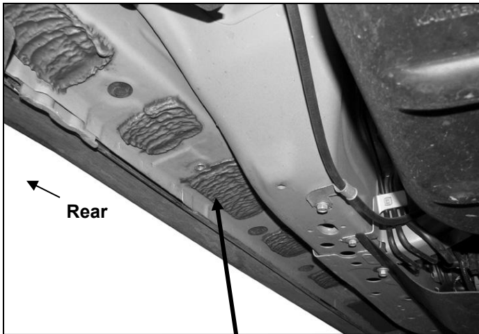
(Fig 12) 8mm Threaded Insert fully installed
