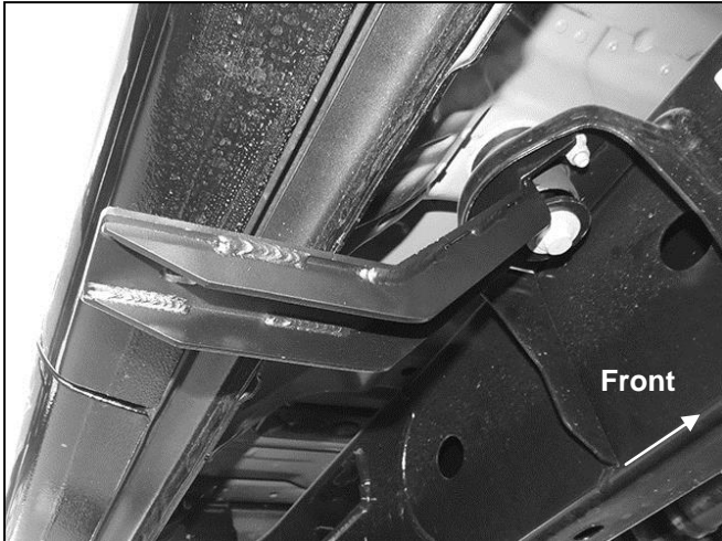
(Fig 7) Passenger/right center Bracket installed
