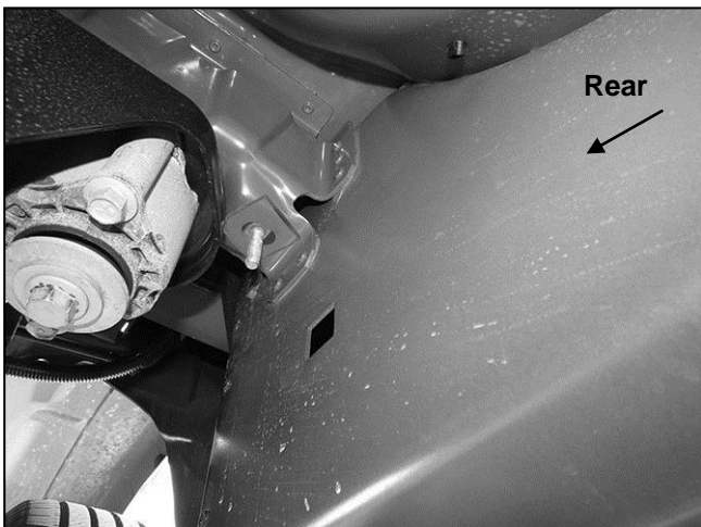
(Fig 11) Insert T-Bolt and folded Washer into oval hole. Thread second Plastic Washer onto T-Bolt
