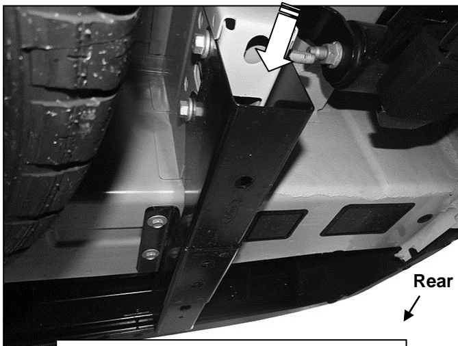
(Fig 1) Driver side mounting location
