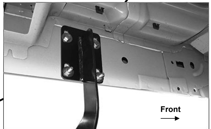
(Fig 5) Front Bracket installation pictured
