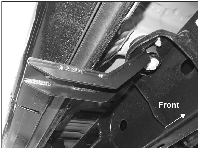
(Fig 7) Passenger/right center Bracket installed
