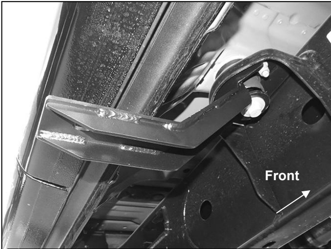
(Fig 7) Passenger/right center Bracket installed
