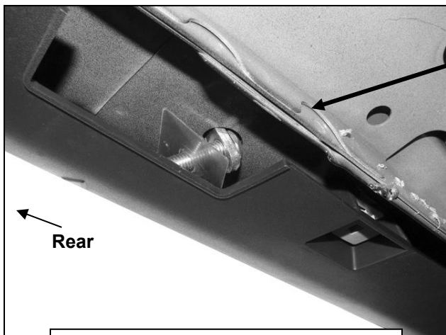
(Fig 16) Rear mounting location with Bolt Plate pictured from below
