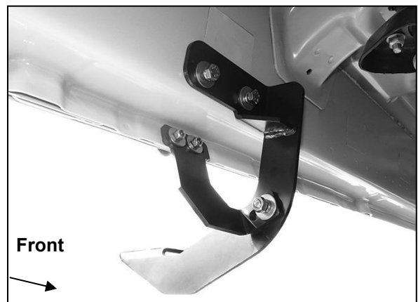
(Fig 14) Attach Driver/Left Support Bracket to back of 2# Mounting Bracket
