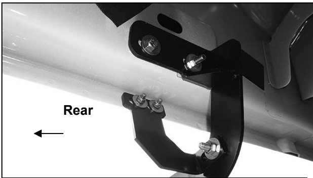
(Fig 17) Driver/Left 3# Bracket assembly
