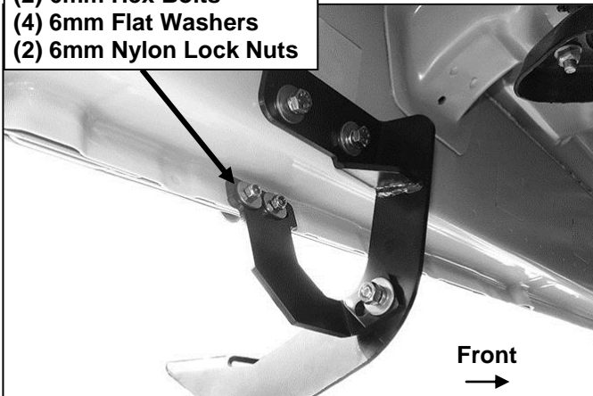
(Fig 11) Driver side front Bracket assembly
